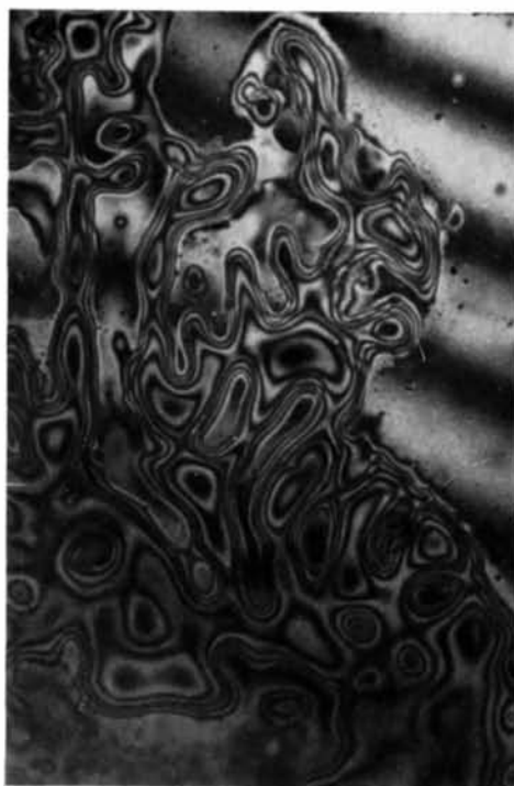
Fig. 4. Unevenness of surface caused by flow in the cholesteric phase of cholesteryl 2-propyn-1-yl carbonate ( \times 150 ).
